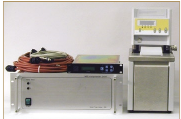
HPM power supply, controllers, cables and heating thermostat for the AKS system
