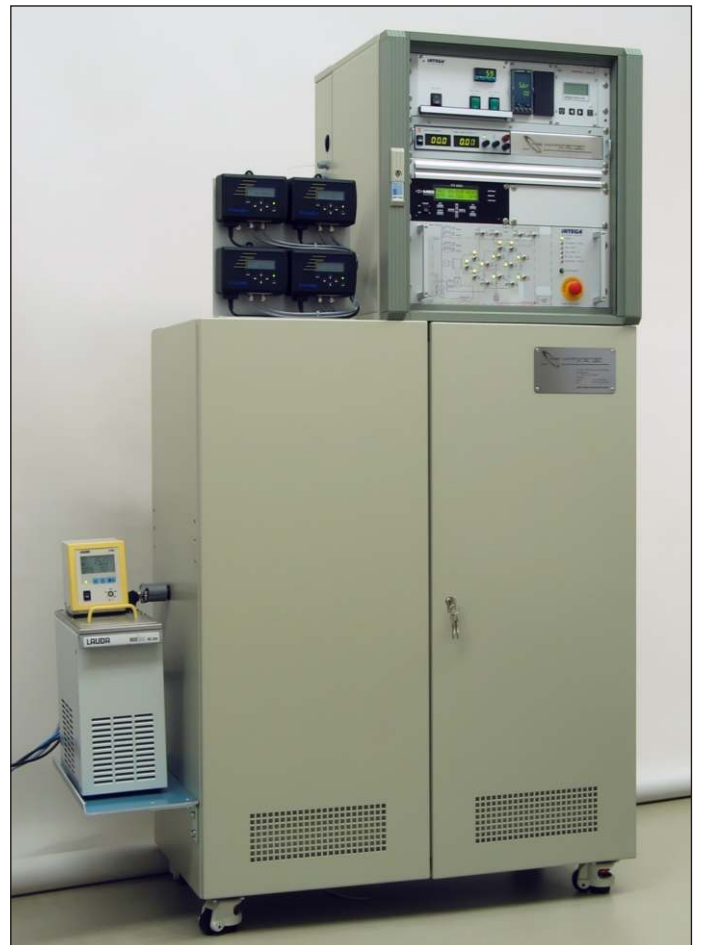
Gas cabinet of the AsBr 3 in-situ etching system ISES
