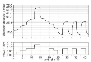
Dynamic behavior of valve operation measured with sulfur
