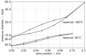
Valve characteristic for  $90^{\circ}\text{C}$  and  $100^{\circ}\text{C}$  reservoir temperature
