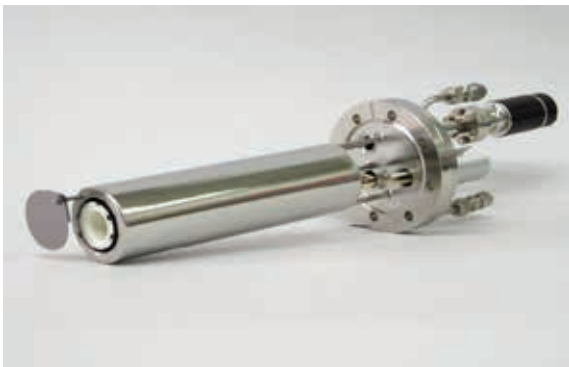
Organic Effusion cell OEZ 63-35-33-S with 35 cm 3 crucible, mounted on a DN63CF (O.D. 4.5") flange, with integrated water cooling and rotary shutter
