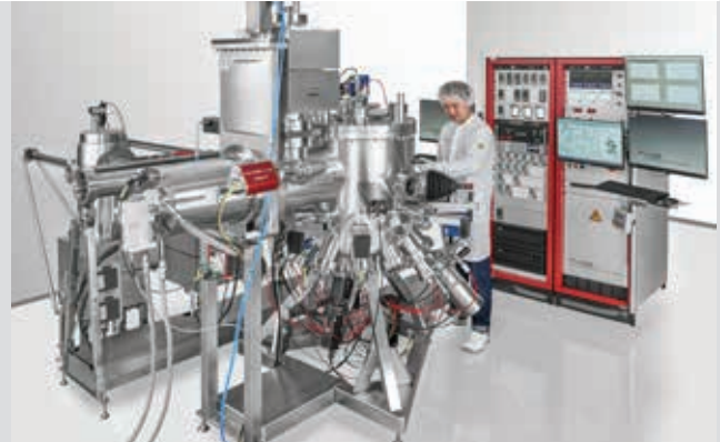
OCTOPLUS 600 MBE system with control rack
