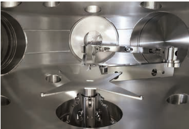
Fully automated wafer transfer by central handling arm.
