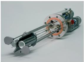
Dual Doping Source DDS 63-2x5-27-S (V80) Two 5 cm³ PBN crucibles with individual cell shutter separated by a water cooling pipe on one flange DN63CF (O.D. 4.5")
