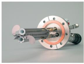
Dual Doping Source DDS 63-2x2-16-S Two 2 cm³ PBN crucibles with individual cell shutter separated by a water cooling pipe on one flange DN63CF (O.D. 4.5") (For RIBER 32 MBE system)
